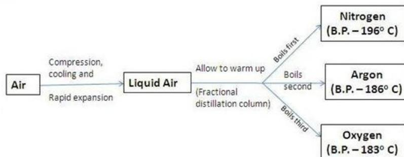
Fig. Separation of major gases of air
